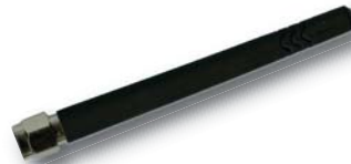
Bluetooth antenna, 2.45GHz, 1/4, 0 dBi, SMA p/n 30-597105-01
